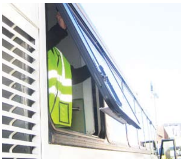
Byron Bloch (left) demonstrates (above) how large swing-out windows in coach restrooms can (and have) suddenly swung open, resulting in passengers falling out onto the road
