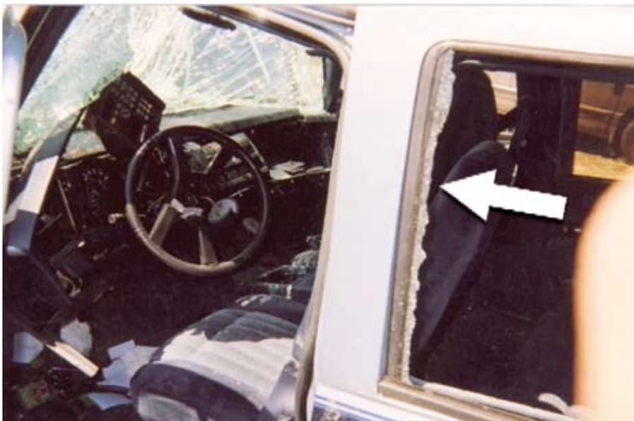
Left: Case A. In this Chevy Suburban SUV, a young girl was seated in the middle row seat, wearing her seatbelt. In the collision, the seatbelt buckle released and she was ejected out through the side window when the tempered glass shattered. The arrow shows glass particles embedded within the rubber molding. Below: IIHS side-impact test of a 2008 Chevrolet Malibu. Note that the laminated forward side glass stays intact, while the tempered rearward side glass shattered completely out.
