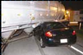
the entire rear of the truck, and side guards must be required on large trucks and trailers with sufficient strength to prevent underride by passenger cars at 50mph-plus in 90° perpendicular crashes. European trucks and trailers are leading the world with sideguards but they must be strengthened and crash-tested to ensure
