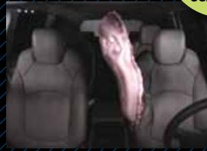
oblique vehicle-to-pole test by simulating a collision sideways into a narrow fixed object, such as a telephone pole or tree. The pole test will be conducted using a 5<sup>th</sup> percentile female dummy seated full-forward, or a 50<sup>th</sup> percentile male dummy seated at the mid-track position of the front outboard driver or passenger seats.
