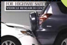
What’s imperative is that countermeasures be designed into the larger vehicles to help soften the impact forces transmitted to the more vulnerable passenger cars.
