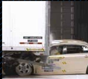
that passenger vehicles will be prevented from the underride hazard. Strengthening can be achieved with additional supports, diagonal braces and gusset plates. US trailers are now slowly adopting side guards, mostly for aerodynamic fuel-efficiency reasons, and they, too, must be made much stronger.
